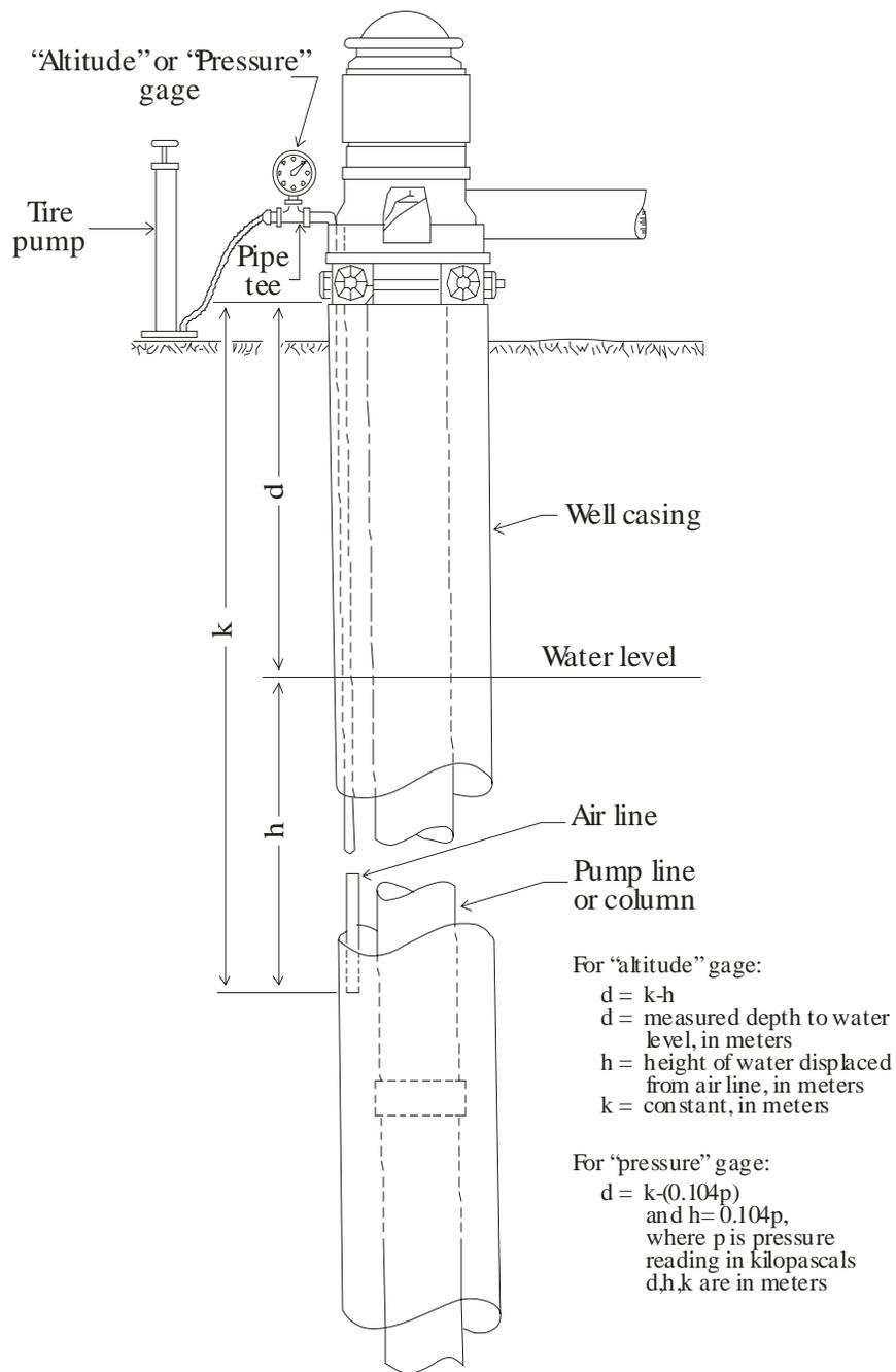
**Figure 3 –Typical installation for measuring water levels by the air-line method and relation of measured depth to water level, height of water displaced from air line, and depth to bottom of air line**
