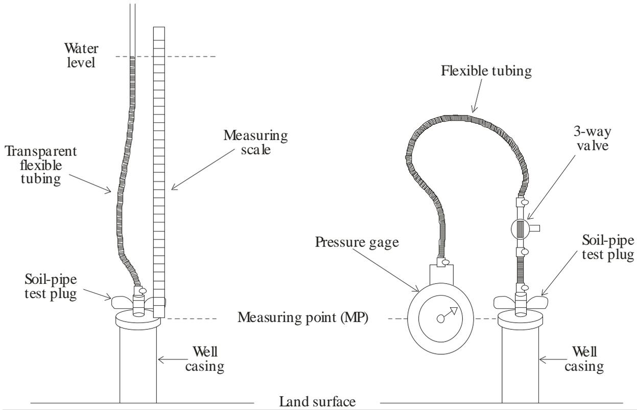
**Figure 4 -- Water level measurement in a flowing well.**
