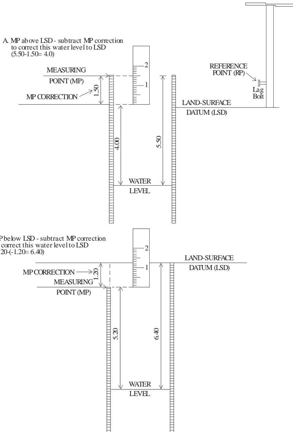
**Figure 5 – Relation of measuring point, (A.) above or (B.) below land surface datum, reference point, and the water level.**
