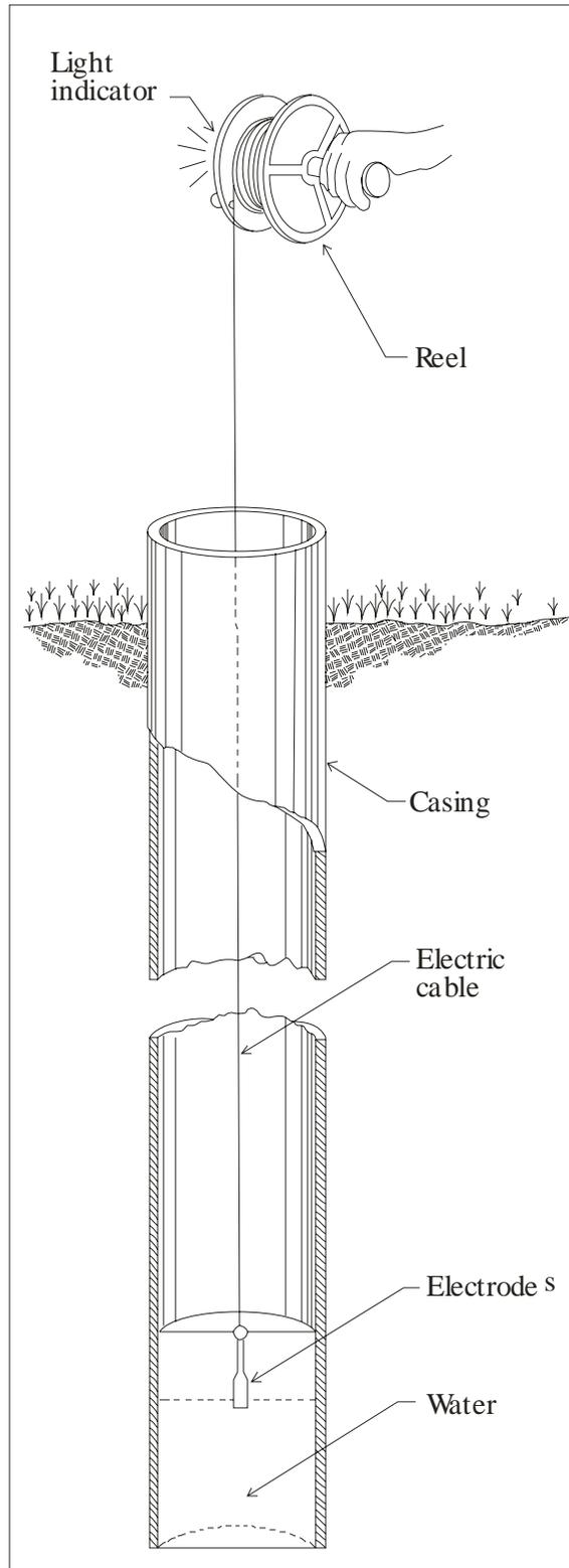
Figure 2 -- Water-level measurements using an electric tape (Driscoll, 1986, fig.16.12)
