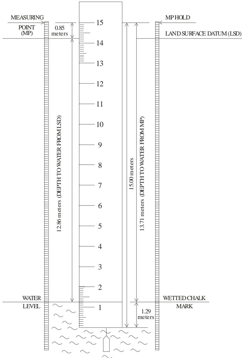
**Figure 1 -- Water-level measurements using a graduated steel tape.**
